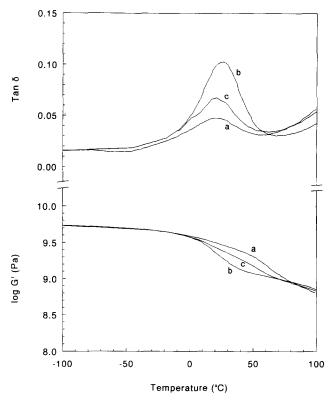
**Figure 10** Dynamic mechanical characteristics *versus* temperature for moulded PHB samples which were (a) stored for 150 days, (b) subsequently annealed for 10 h at 110°C, and (c) stored for another 150 days
