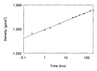
Figure 11 Density changes at 25°C as observed by dilatometry in a sample which was annealed at 110°C for 10 h
