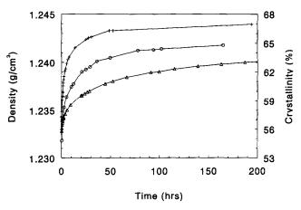
Figure 8 Density changes in as-moulded PHB as observed by dilatometry at 25°C (△), 43°C (○), and 60°C (+)
