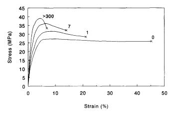
Figure 2 Stress-strain curves at ambient conditions for moulded PHB samples after different periods of storage. The storage times, in days, are indicated in the curves
