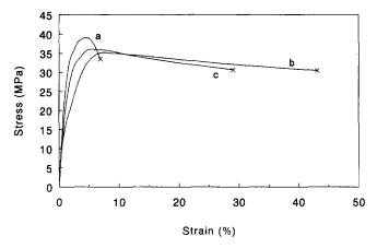
Figure 9 Stress-strain curves at ambient conditions for moulded PHB samples which were (a) stored for 150 days, (b) subsequently annealed for 10 h at 110°C, and (c) stored for another 150 days
