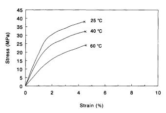
Figure 7 Stress-strain curves at different temperatures for moulded PHB samples which were stored for 400 days
