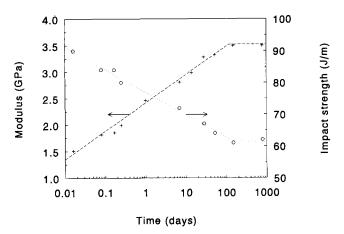
Figure 3 Tensile modulus (+) and Izod notched impact strength ( $\bigcirc$ ) of moulded PHB versus storage time
